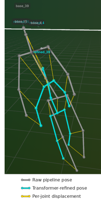
Figure 8: Qualitative comparison of a single player pose before and after Transformer refinement. The deterministic pipeline output after Stage 4 is shown in grey, the refined output in cyan, and yellow lines connect corresponding joints to indicate the magnitude and direction of the per-joint correction. The displacement is largest at the extremities and smallest near the torso, consistent with the proximal-to-distal error gradient reported. The refined skeleton is also smaller overall, reflecting the correction of the pipeline’s tendency to over-scale players.
