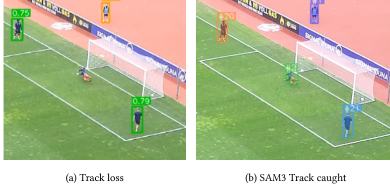
Figure 3: Failure modes observed in YOLO-based detection [28] applied to broadcast football footage. (a) The goalkeeper is dropped entirely by the tracker despite remaining clearly visible in the frame, caused by a confidence drop induced by an atypical player posture. (b) SAM 3 successfully re-acquires and tracks the same player correctly. Together, these failure modes motivate the adoption of the SAM 3-based segmentation pipeline introduced in Section 4.2.
